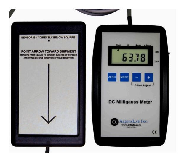
This meter is used to verify compliance with IATA, IACO and FAA regulations on magnetism from packages to be shipped by air.\*
