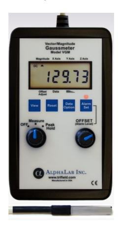
Displays X,Y,Z and magnitude of magnetic field, for rapid mapping and measurement of magnetized materials. Range is 799.99 gauss.
