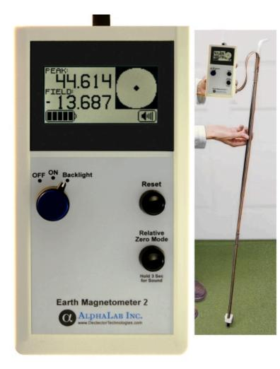
The Earth Magnetometer Model EM2 measures the Earth magnetic field with a resolution of 1nT (1 gamma). This resolution is about 0.002% of the typical Earth field strength. It is used to locate buried magnetic objects or materials.
