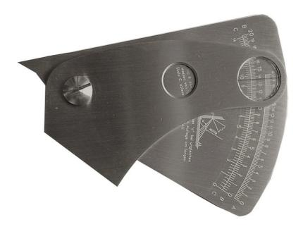
Designed to measure fillet weld: weld height, leg length of a fillet weld
