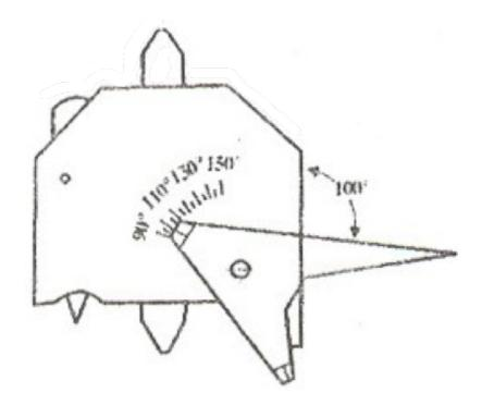
Measure width of the weld: close up the main measuring angle to one side of the weld firstly; then rotate the measure angle of the multi-purpose gauge to close up to the other side of the weld; and see the indicating value of the multi-purpose gauge for the width of the weld (Diagram 6).
