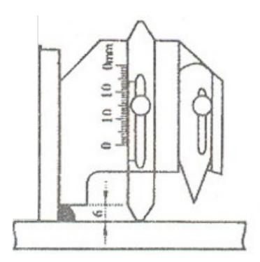
Measure the fillet weld: the welding spot at 45 degrees is the thickness of the fillet weld. First close up the working face of the main body to the weldment; move the height gauge to touch the welding spot; and see the indicating value of the height gauge for the thickness of the fillet weld (Diagram 3).
