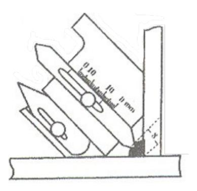
Measure the undercut depth of the weld: first align the height gauge to zero and fix the screw; and use the undercut gauge to measure the undercut depth and see the indicating value of the undercut gauge for the undercut depth (Diagram 4).
