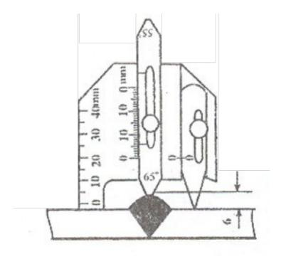
Measure the height of a fillet weld: move the height gauge to touch the other side of the weldment and see the indicating line of the height gauge for the height of the fillet weld (Diagram 2).
