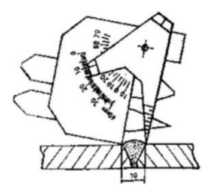
Measure a fit-up gap: insert the multi-purpose gauge between two weldments; and see the indicating value of the gap gauge on the multi-purpose gauge for the gap value (Diagram 7).
